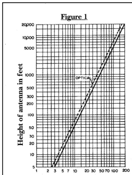
This diagram can give you an idea of the line-of-sight distance. To use it compute the distance for the height of the transmitter and your own height separately, then add them together. For example, if your transmitter was on a hill 25 feet high and your receiver was 8 feet high, the line-of-sight distance would be 11 miles (7 + 4 miles).
