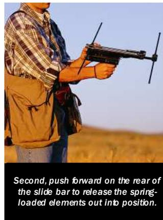
*Second, push forward on the rear of the slide bar to release the spring-loaded elements out into position.*
