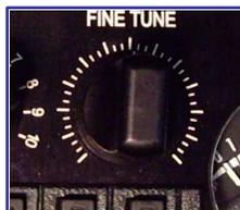
The **Fine Tune Knob** is available so you can adjust the frequency slightly (within one KHz.) The tuning is very broad and not "touchy."
