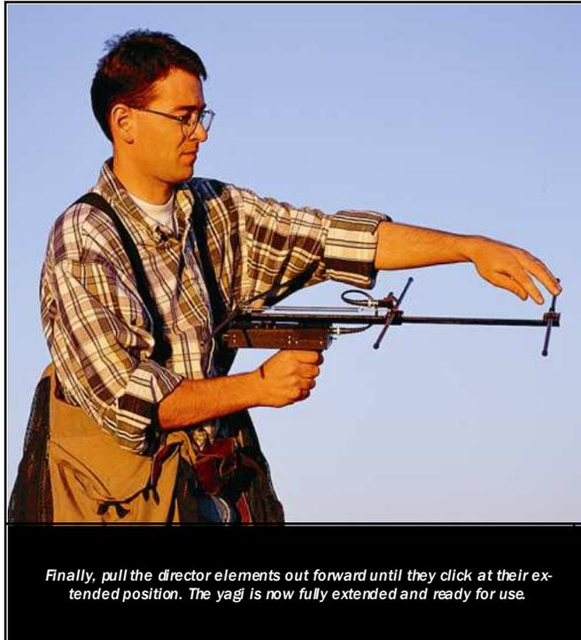
**REMEMBER!** The antenna won't give its best range and pin-point accuracy **unless fully deployed** as shown in the picture above.
