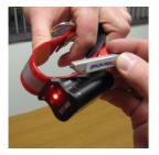
**Turn** the *High Intensity* Lights on/off, tap the light bulb symbol (located on the back side of the collar) with the magnet (Transmitter must be running before you can active the Lights).
